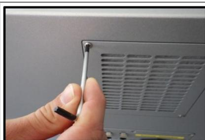
Remove the four screws using a TX20 Torx key.
