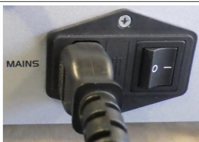
Reconnect the mains plug and set the mains switch back to position 1.
