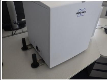
Unscrew the handles using an Allen key and remove them from the spectrometer.
