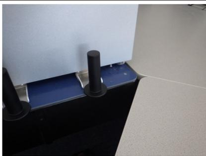
Move the pallet to the edge of the table and set it flush with the edge of the table and pallet edge, activate the parking brake of the lift truck.
