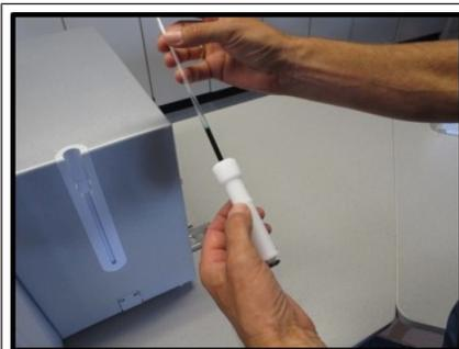
Insert the sample into the sample holder from above.
