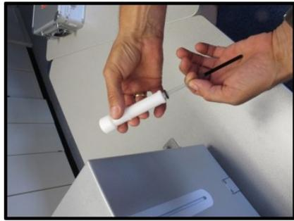
Continue to gently pull the sample down until a slight resistance is felt. Do not go too far, as this may push the cap out so that it hangs in the spinner.
