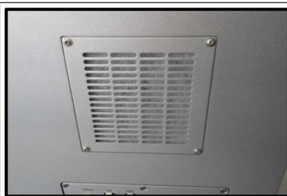
Filter grill on the back of the electronics unit above the connection panel.
