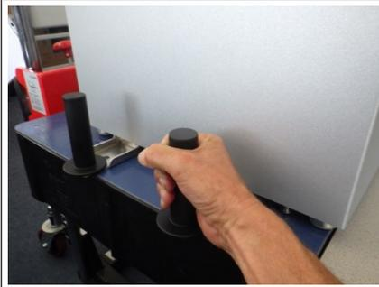
Carefully slide the spectrometer onto the table using the handles located on the bottom of the spectrometer.
