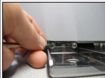
Remove the transport plates using the Allen key.
