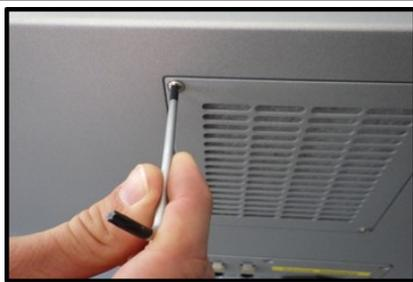
Tighten the four screws using a TX20 Torx key.
