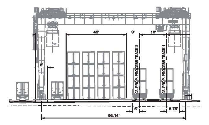
RTG CRANE TYPICAL SECTION
