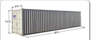
40 ft. High-Cube Container Dimensions Approximate interior dimensions: 39' X 7'8" X 8'9" Payload: 64,270 lbs. Tare weight: 8,930 lbs. Cubic capacity: 2,681 cu. ft.
