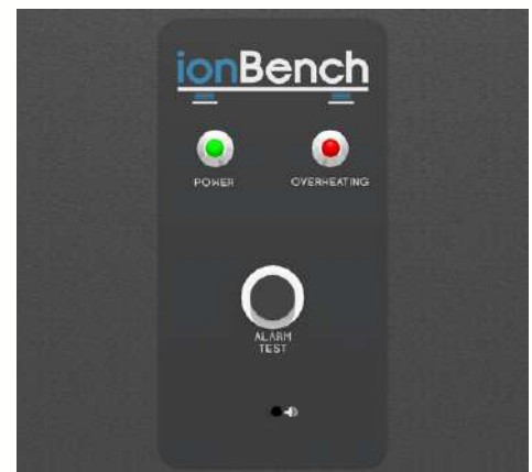
Overheating temperature alarm
